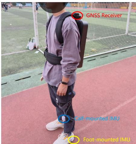
Fig. 4: The relative positional relationship between foot-mounted IMU, shin-mounted IMU, and GNSS receiver.
