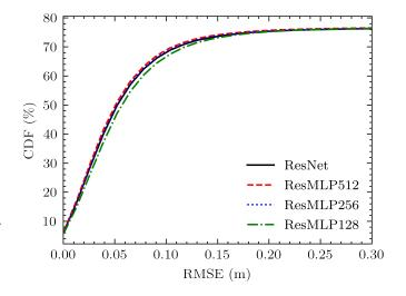
Fig. 4. Comparison of the inference error CDFs of different models in the test set. The network infers the displacement in 1 second as described before.
