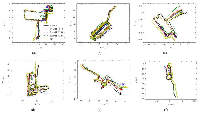
Fig. 6. Selection of trajectories with different contours. The ground truth trajectory generated from the Tango phone denoted as GT and marked in yellow. The ResNet trajectory is denoted by the black line. The ResMLP512, ResMLP256, and ResMLP128 are represented by red, blue, and green, respectively.
