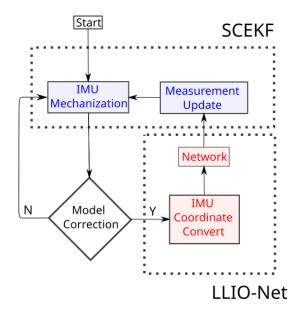
Fig. 1. System flowchart. The block named model correction selects a keyframe for inference displacement based on LLIO-Net. In this paper, the key frame is selected every 0.1 s.
