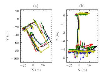
Fig. 7. Selected trajectory with height illustrated. (a) illustrated trajectory in the x-y plane. (b) illustrated trajectory in the x-z plane. The ground truth trajectory generated from the Tango phone is denoted as GT and depicted in yellow. The black line represents the ResNet trajectory. The ResMLP512, ResMLP256, and ResMLP128 are represented in red, blue, and green, respectively.
